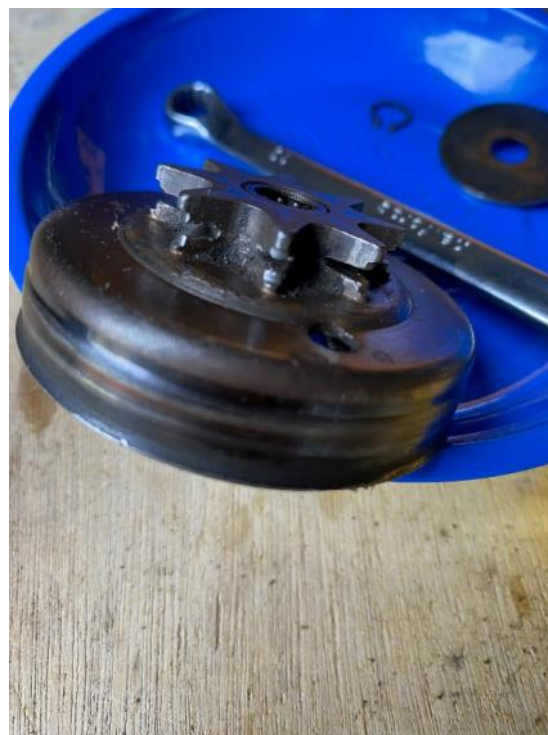
and the sprocket – with the teeth almost cut in half by the old chain
